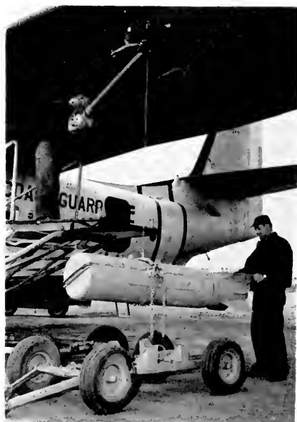
FIGURE 16.—U.S. Coast Guard UF-2G amphibian aircraft being armed with 1,000 pound incendiary bomb cluster in preparation for iceberg demolition experiment.
